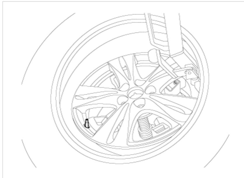
4. After bottom bead is on tire, rotate the rim until the valve is at the 5 o'clock position relative to the head on the tire changing machine. Push down on the tire at the 3 o'clock position and rotate the rim clockwise to fit the top bead.
