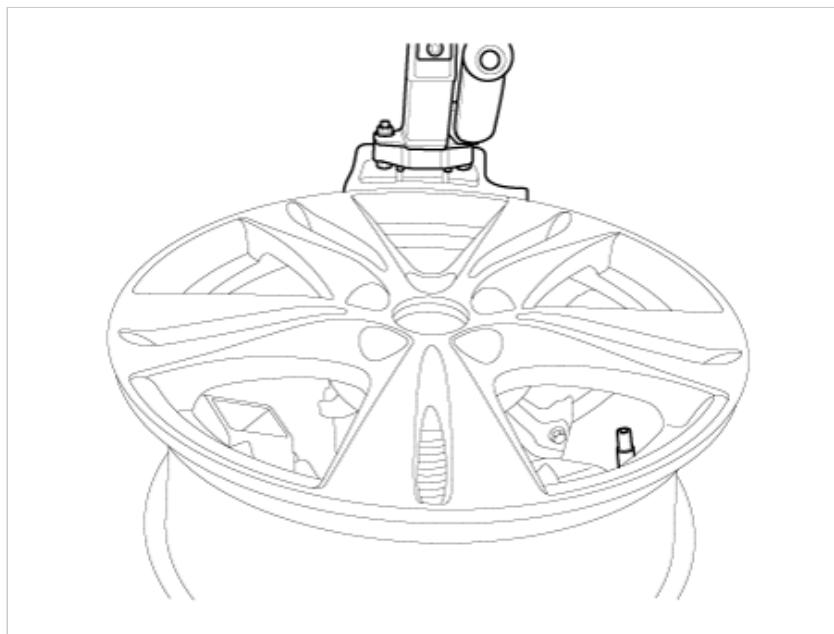
3. Place the tire on the rim so the bottom bead touches the edge of the rim after the valve (6 o'clock). Rotate the rim clockwise, and push down on the tire at the 3 o'clock position to fit bottom bead.
